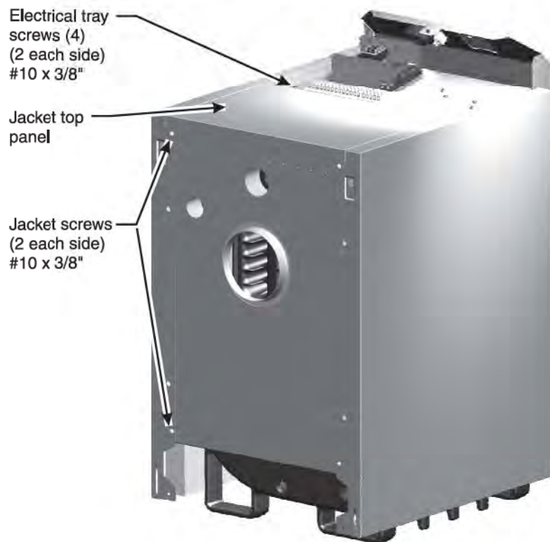
Figure 20 Jacket components and hardware
