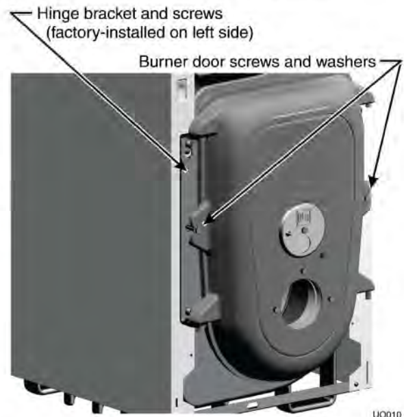
Figure 4 Burner door hinge installation
